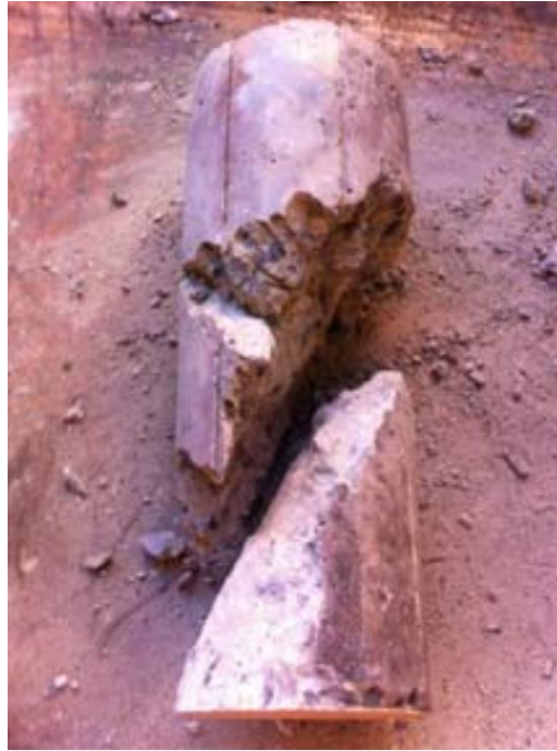
Fig. 3 A column fail due to concentric load with a single sliding plane
