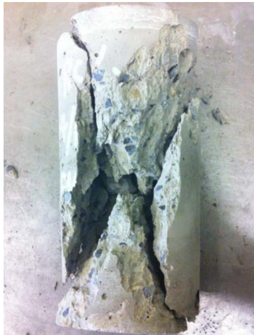
Fig. 4 A column fail due to concentric load with a circumferential wedge
