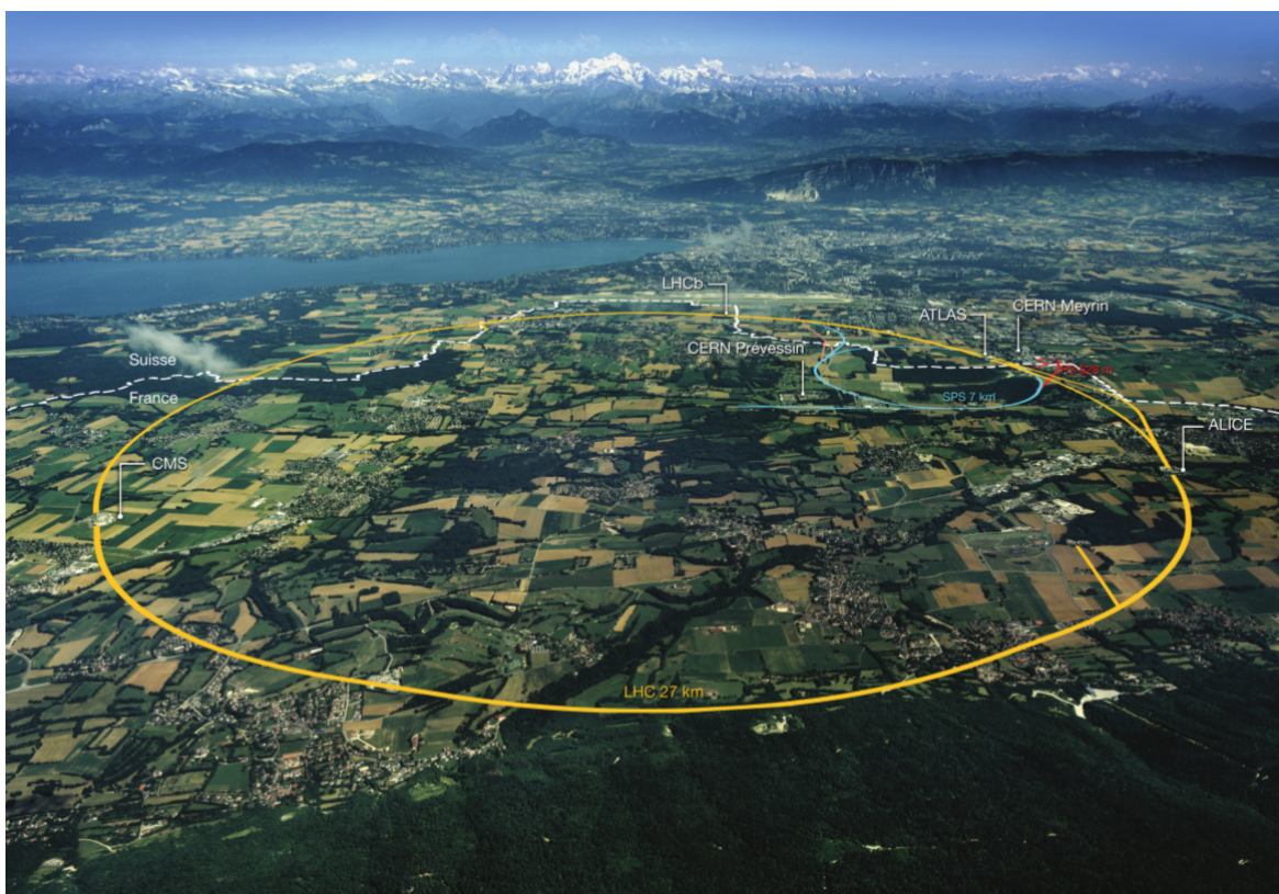
Fig. 3.2 An image showing the locations of major sites, detectors and accelerators overlaid on an aerial photo showing the area around Geneva. Photo taken from the CERN 60 Year Anniversary Celebration [32]. The RED circle represents the Proton Synchrotron, the BLUE circle represents the Super Proton Synchrotron and the YELLOW circle represents the Large Hadron Collider.
