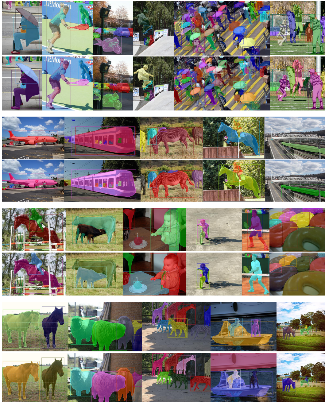
FIGURE 4.5. Selected results of Mask R-CNN (top) and BlendMask (bottom). Both models are based on Detectron2. The Mask R-CNN model is the official 3\times R101 model with 38.6 AP. BlendMask model obtains 39.5 AP. Best viewed in digital format with zoom.
