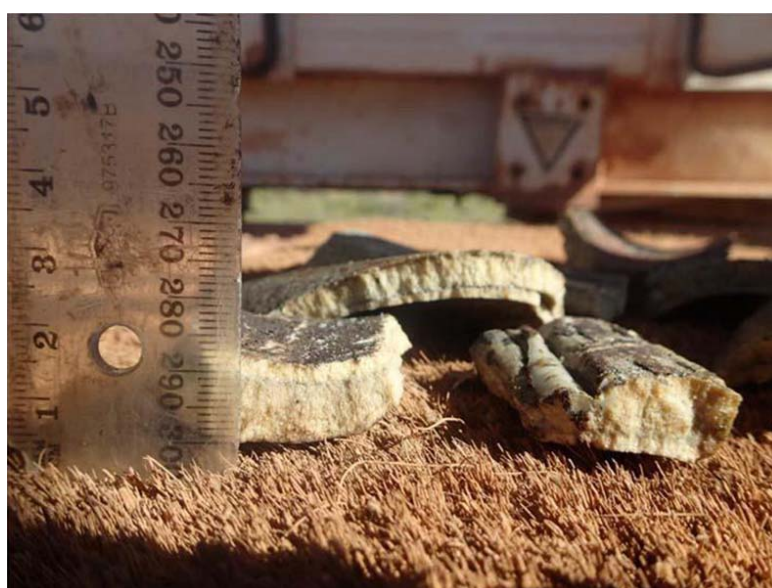
Fig. 5—Scale removed from perforations after scraper run during workover.
