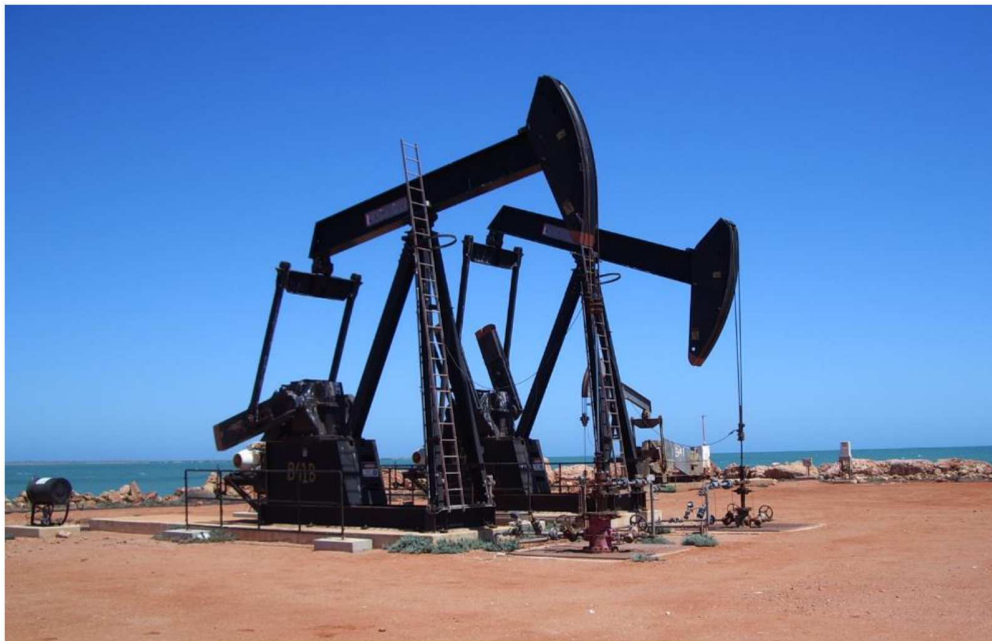
Figure 6—Photograph of B41B and B41C beam pump units, producing from the Windalia formation
