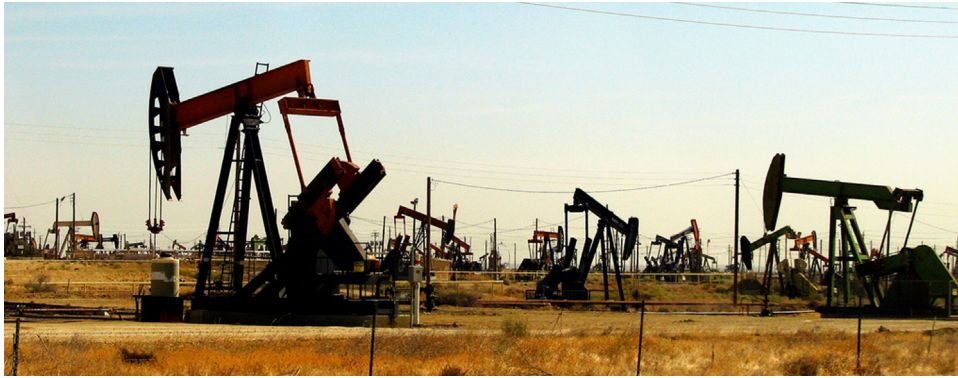
Fig. 1. Sucker Rod Pump units and POCs in California, United States (Photo by Colin G Palmer/Creative Commons).
