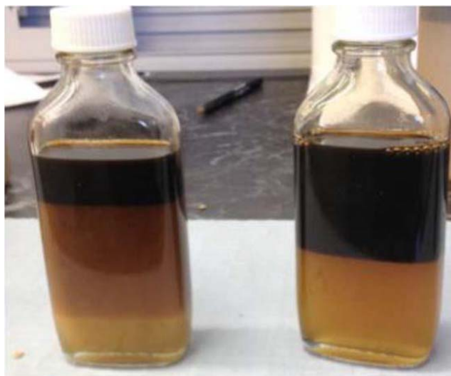
Fig. 10—Emulsion testing of Windalia fluid sample with acid recipe (qualitative method). Sample on the left has settled for 2 minutes; sample on the right settled for 30 minutes.
