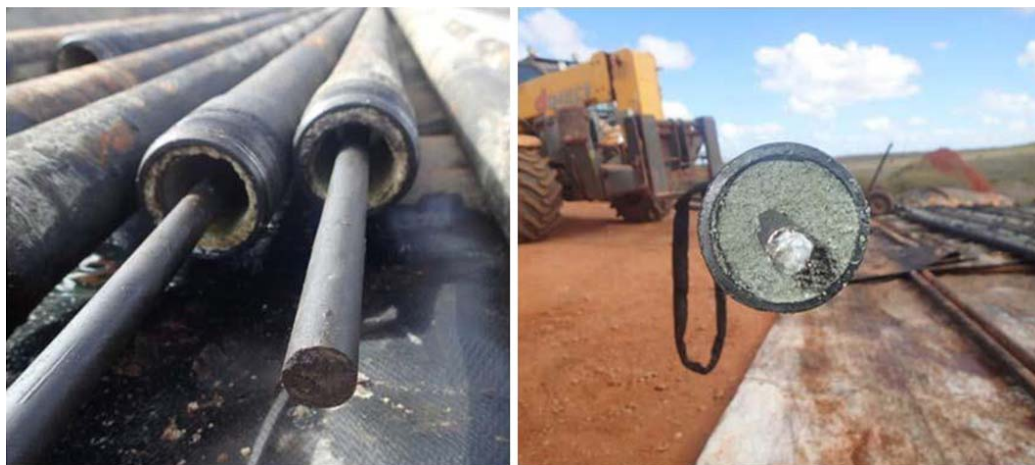
Fig. 4—Scale observed in tubing (left) and sucker-rod-pump plunger (right).
