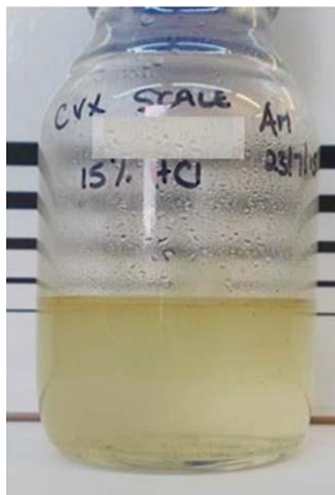
Fig. 12—HCl testing of 1-g scale sample, dissolving within 1 minute (well name removed). A small amount of scale was added to the 15% HCl solution. Gas evolved rapidly and the 1-g scale sample dissolved completely.
