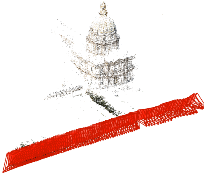
FIGURE 1.4: A demonstration of SfM, where each “ red prism ” denotes the position of the camera centre, and each “ dot ” denotes the reconstructed 3D points.
