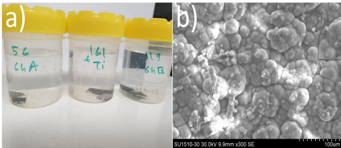
Figure 3.6. a) Samples during SBF mineralization test, b) Typical SEM image of the surface after mineralization process for 21 days.
