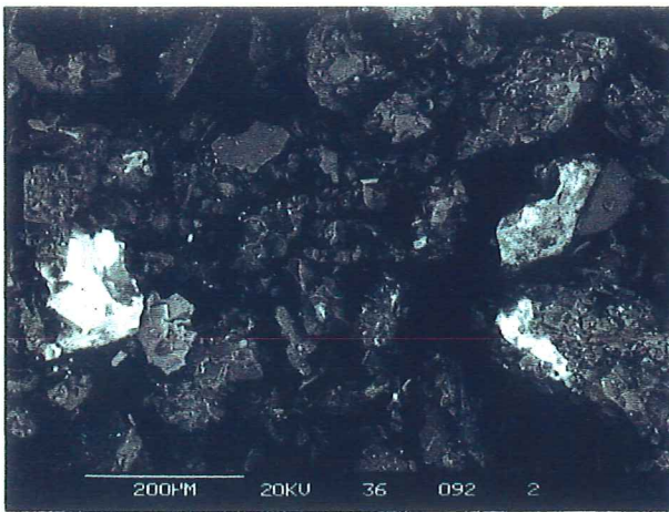
Fig 3C.23 Tailings within zone B, ie below main oxidised zone, 1.47-1.48m depth, larger quantities of sulfides, with little or no oxides present.
