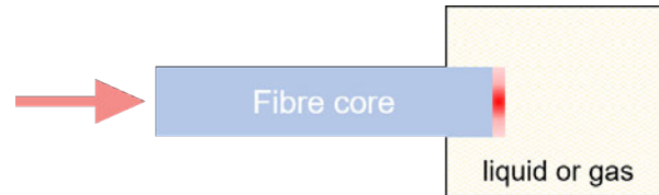
Fig. 2.6 Illustration of a fibre-tip sensor for detecting the surrounding environment, which are generally gases or liquids.
