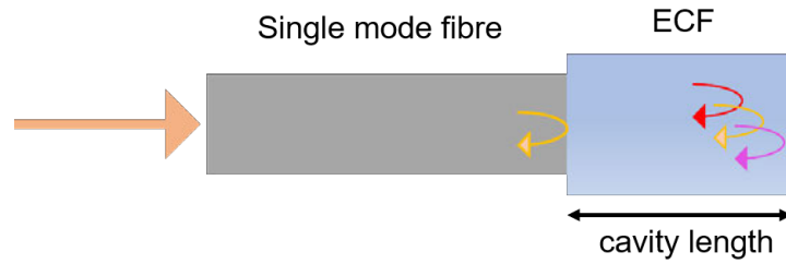
Fig. 3.8 An illustration of a single mode fibre (SMF) spliced to an ECF, where a few modes from the ECF are excited and reflected back to interfere with the reference light reflected from the splice between the SMF and the ECF.
