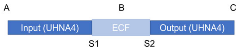
Fig. B.1 An illustration of the splicing configuration, where S1 is the ECF input splice location while S2 is the ECF output splice location.
