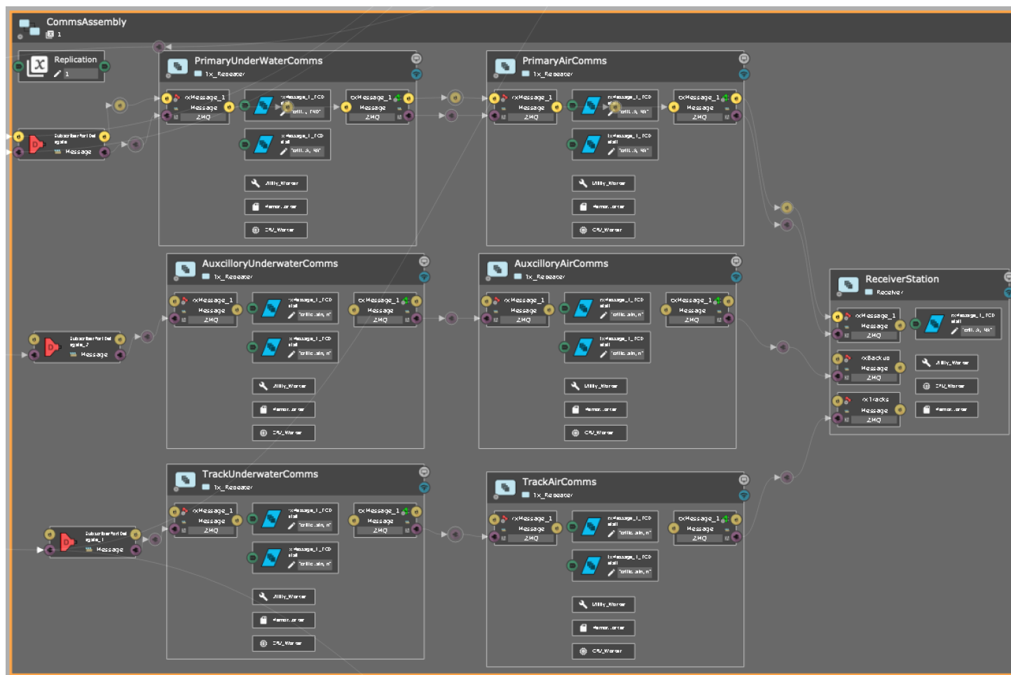
Figure 7.7: MEDEA assembly view of undersea sensor software system CommsAssembly Assembly
