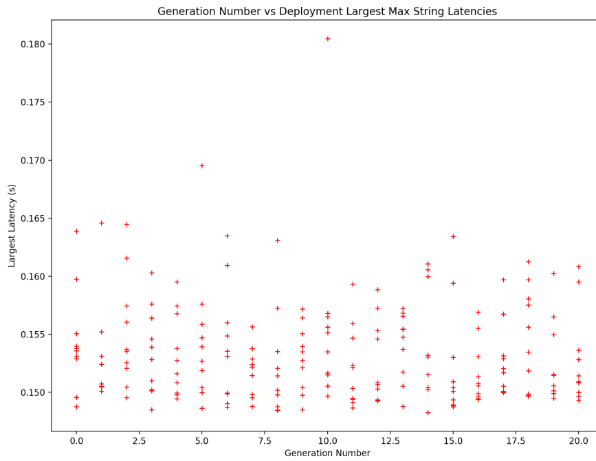
Figure 6.22: Largest measured string latencies for a 130ms modelled defined constraint
