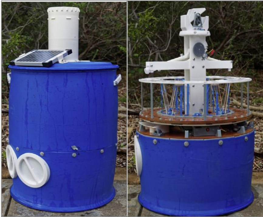
Figure I. Automated rainfall sampler (Ankor et. al. (2019), installed at Wannan water treatment plant, McArthur
