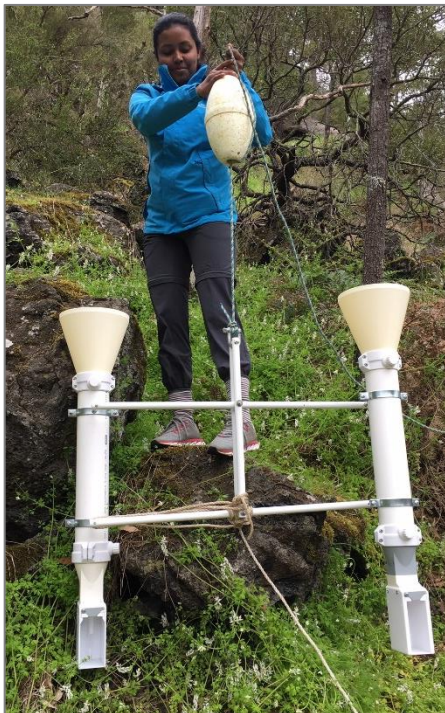
Figure II. Lake sediment trap used to collect sediment samples from the lake bottom. Each end collects two 125 ml sediment column
