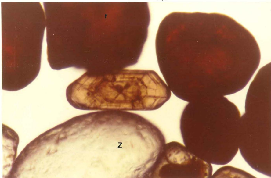
4. Zircon (z) and rutile (r). Note the yellow, euhedral, zoned metamict zircon.
