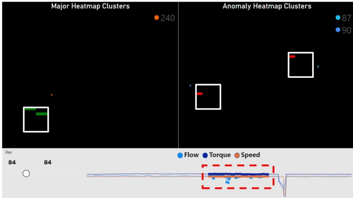
Fig. 37 Day 84 of PCP operations with the selected abnormal behaviour and the respective major and anomaly heatmap clusters
