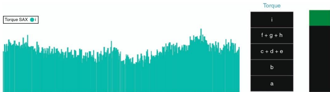
Fig. 11. Torque time-series data conversion to SAX HEATMAP. Symbol (i) is colour coded green.
