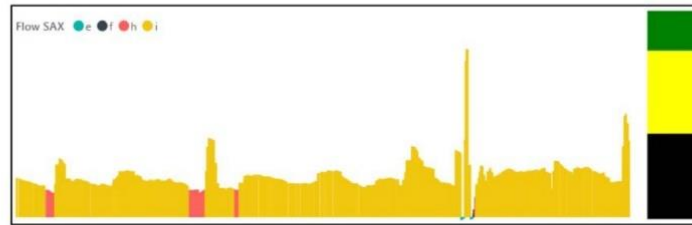
Figure 11—Flow Time Series Data conversion to HEATMAP Image
