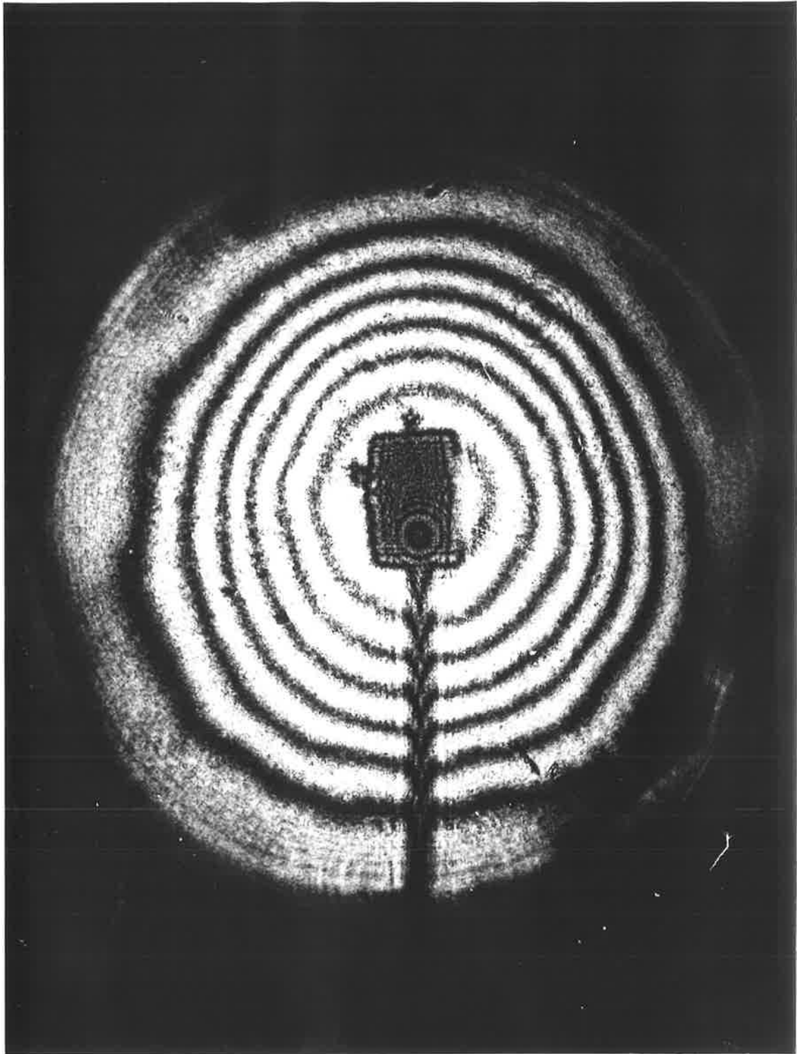
Figure 3.16: An interferogram of the corrected aperture imaged to the plane of the mirror surface ( c.f. uncorrected image in Figure 3.11). This is the diffracted beam, after the lens train.
