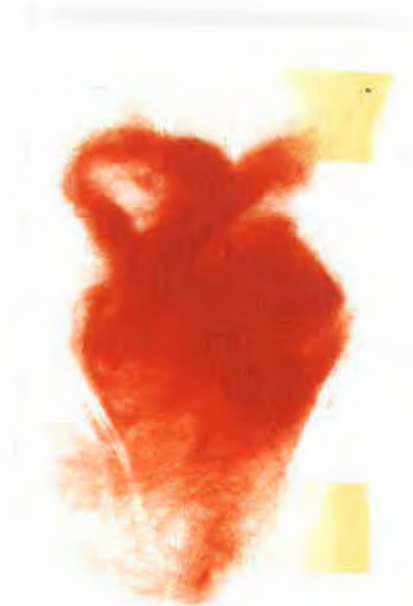
Sample B: Wool treated with 0.1 M thioglycolic acid
