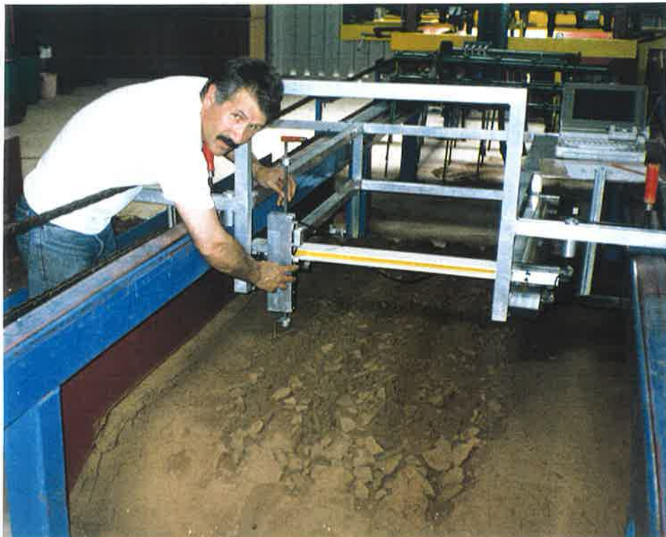
Figure 4.3 Photograph of the seed locations and soil profiles measuring frame.
