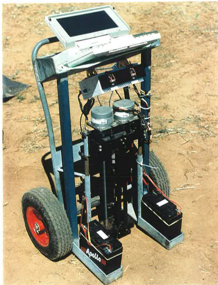
Figure 5.1 Photograph of the motorised pnetrometer.
