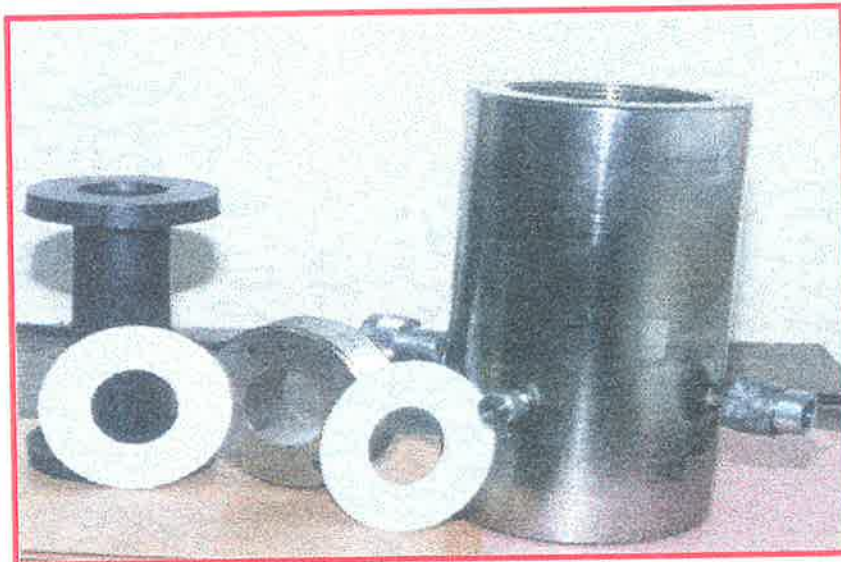
Figure 5.3. Dismantled ITR high-pressure Hoek cell.
