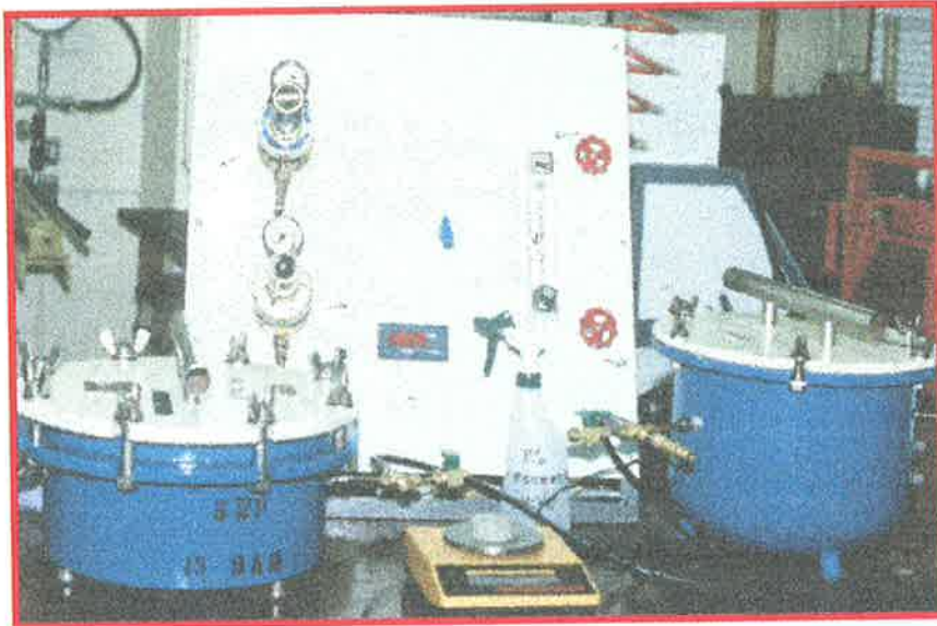
Figure 5.5. Photograph of pressure vessels used for the porous plate extraction technique.
