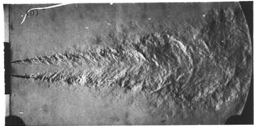
Fig. 3.14 Shadowgraphs of a two-dimensional jet flow ( \rho_J/\rho_0 = 0.57 , \nu = 5.1 \times 10^{-5} , Re = \frac{UD}{\nu} ; (A) 4.0 \times 10^2 ; (B) 4.0 \times 10^3 ; (C) 1.27 \times 10^4 ; (D) 6.0 \times 10^4 )
