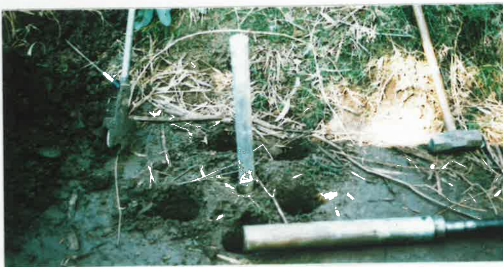
Plate 7.3 In-situ calibration sampling around a neutron moisture meter access tube by augering to the selected depth and driving a sampling tube.
