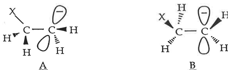
Figure 2.4 Conformers of a \beta -substituted ethyl anion in which the hyperconjugation effect is maximised ( A ) and minimised ( B ).
