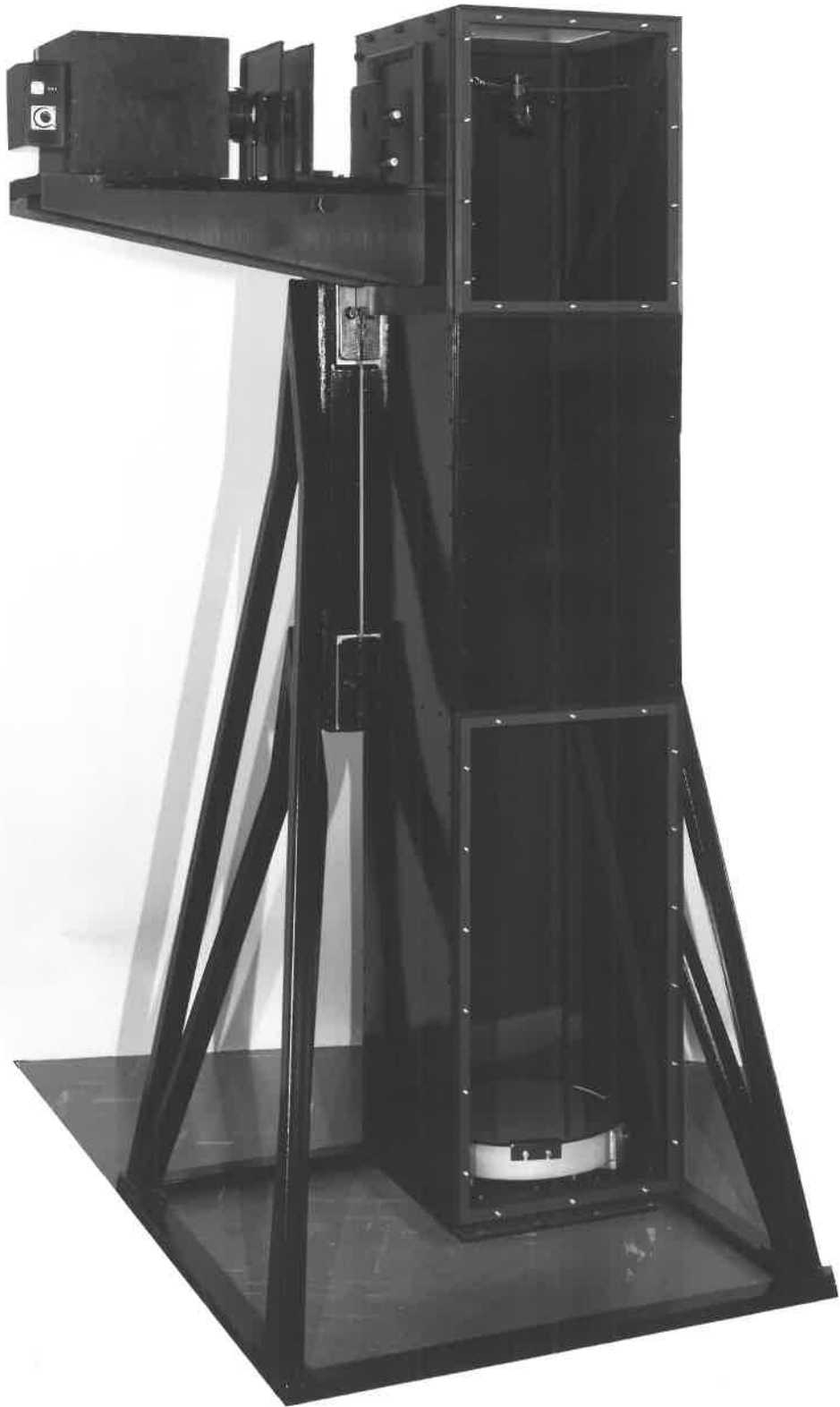
Figure 4.3 Optical receiver with covers removed.
