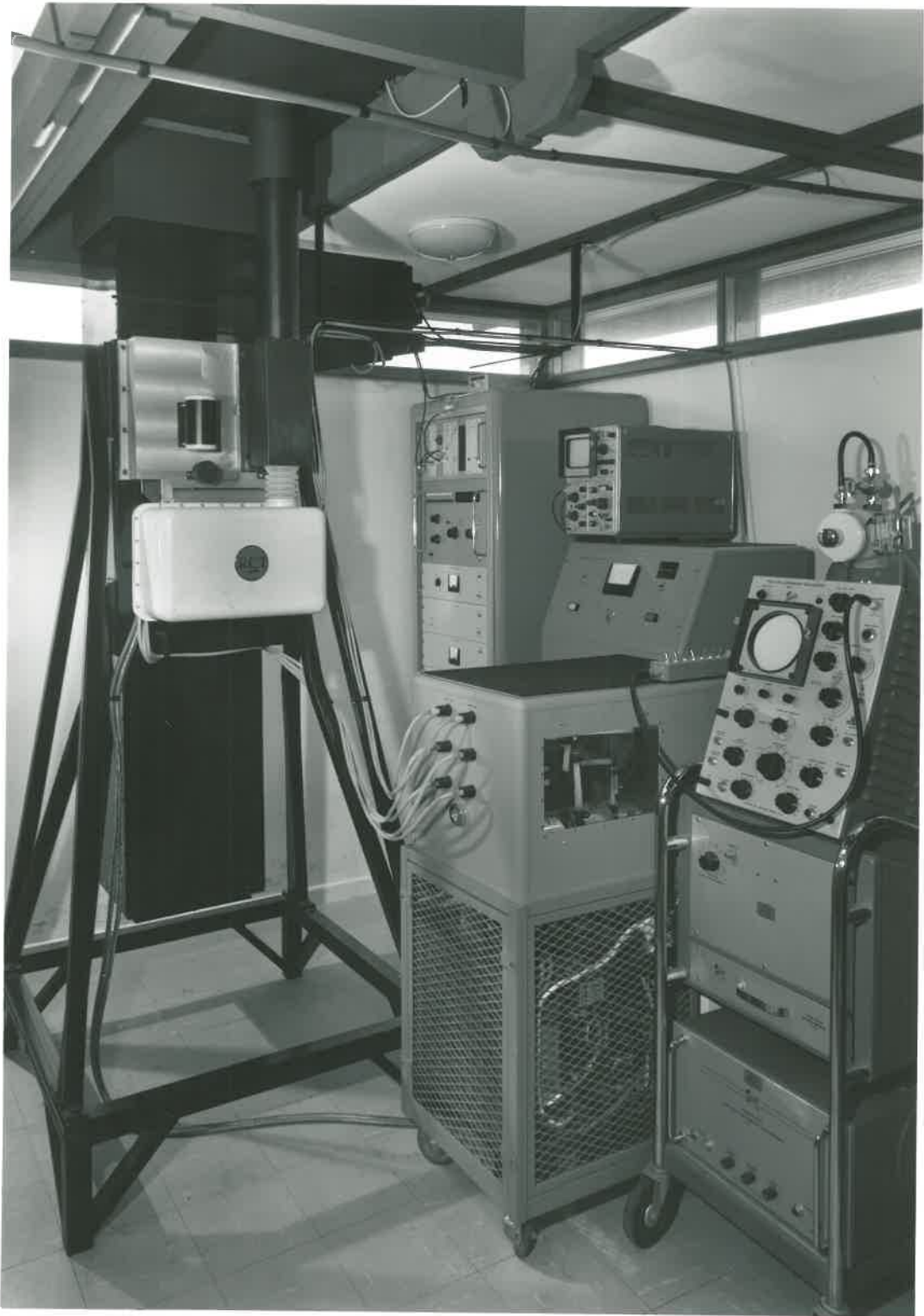
Figure 4.10 Laser radar installed at the field station.
