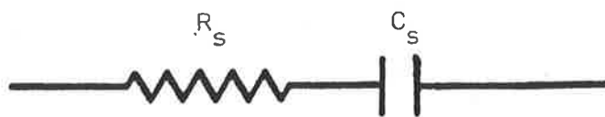
Figure 1a. Simple model of the electrode/electrolyte solution interface consisting of a capacitor and resistor in series.
