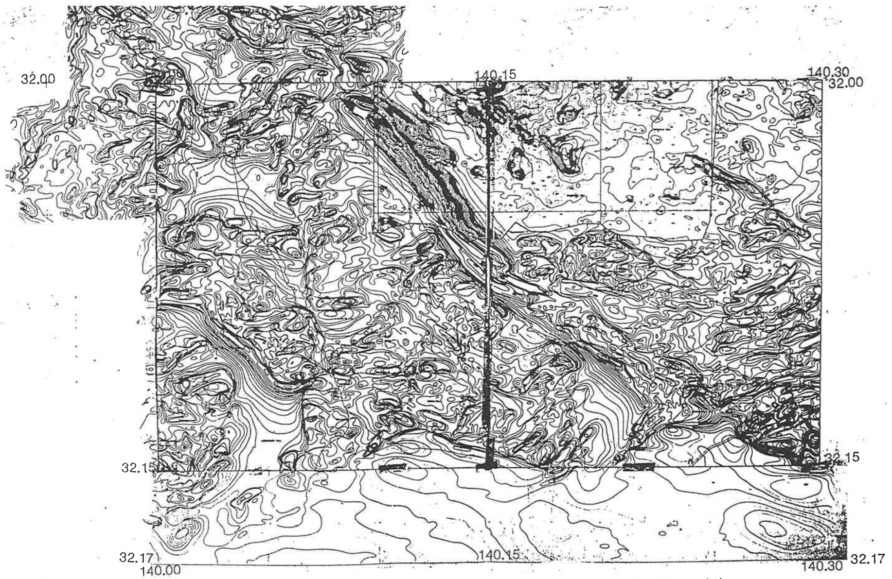
Figure 4.2 The aeromagnetic map of the Olary Province (photo reduced version of the 1:50,000 contour map).
