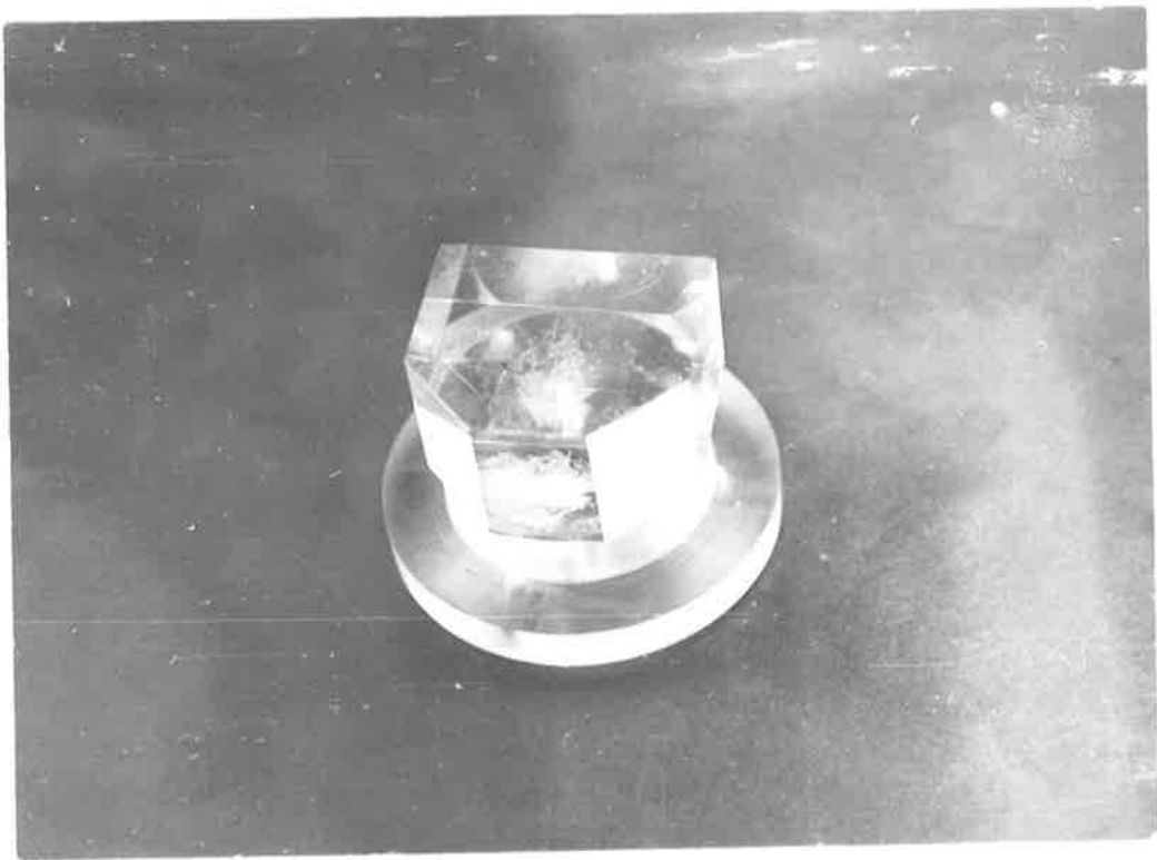
Photo. (2-IV). The perspex block used as a calibration constant in the turbidimeter.
