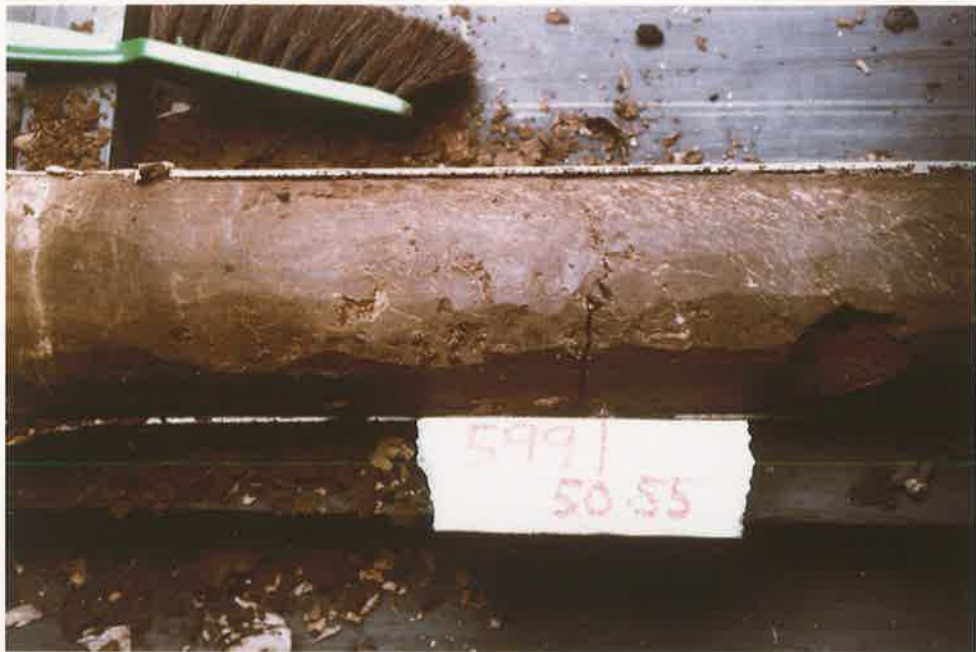
Plate 5.7 Top of CN1 - Near vertical extension joint in sandy silt infilled with fine light brown sand (core diameter = 10 centimetres, top of core to the right).
