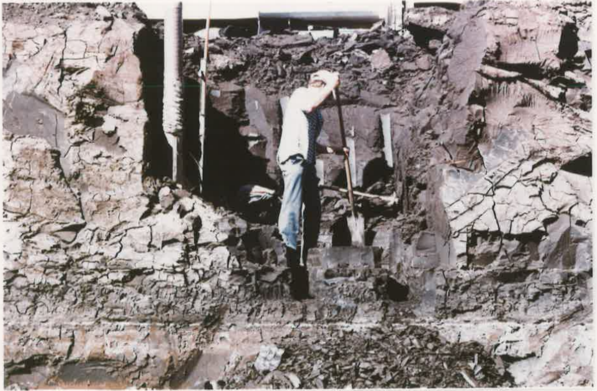
Plate 6.38 Sampling of Tarella Silt Shear Zone or shear testing.
