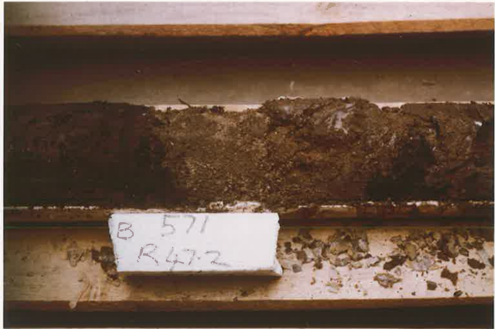
Plate 5.1 Sharp erosional contact between a clean sand facies and a carbonaceous silt facies. Note the large clay gall and piece of wood lying at the base of the sand facies (core diam. = 10 centimetres, top of core to the right).
