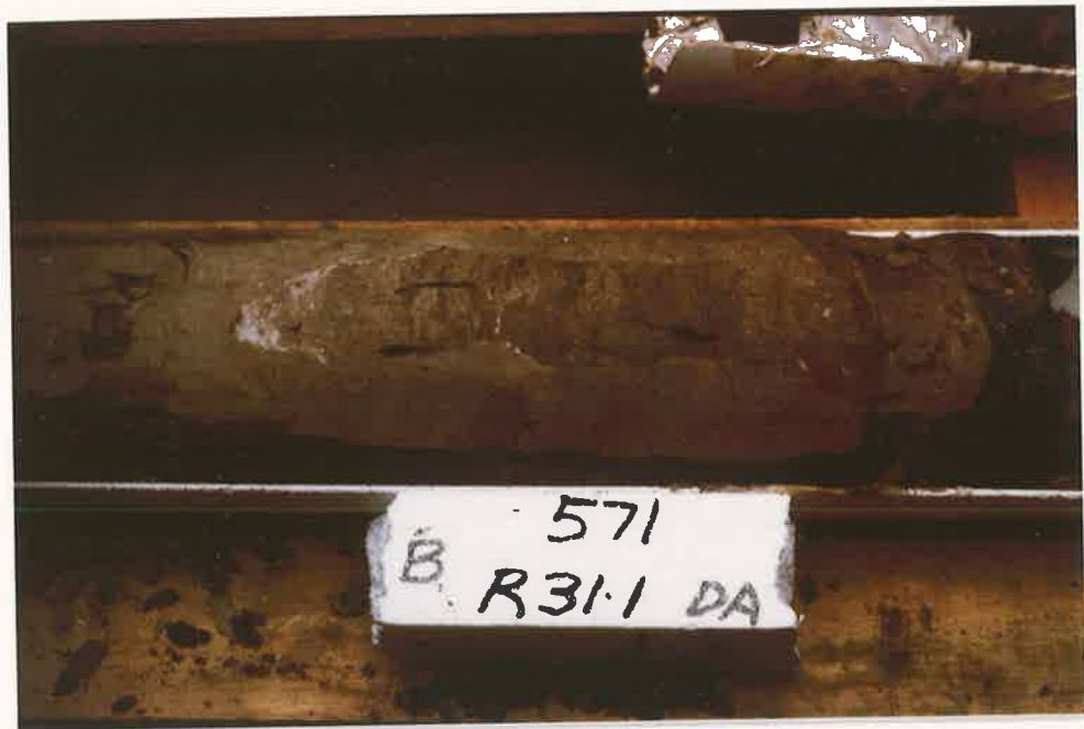
Plate 5.5 Top of the Darnleigh Park Sand Member exhibiting a large infilled burrow (core diameter = 10 centimetres, top of core to the right).
