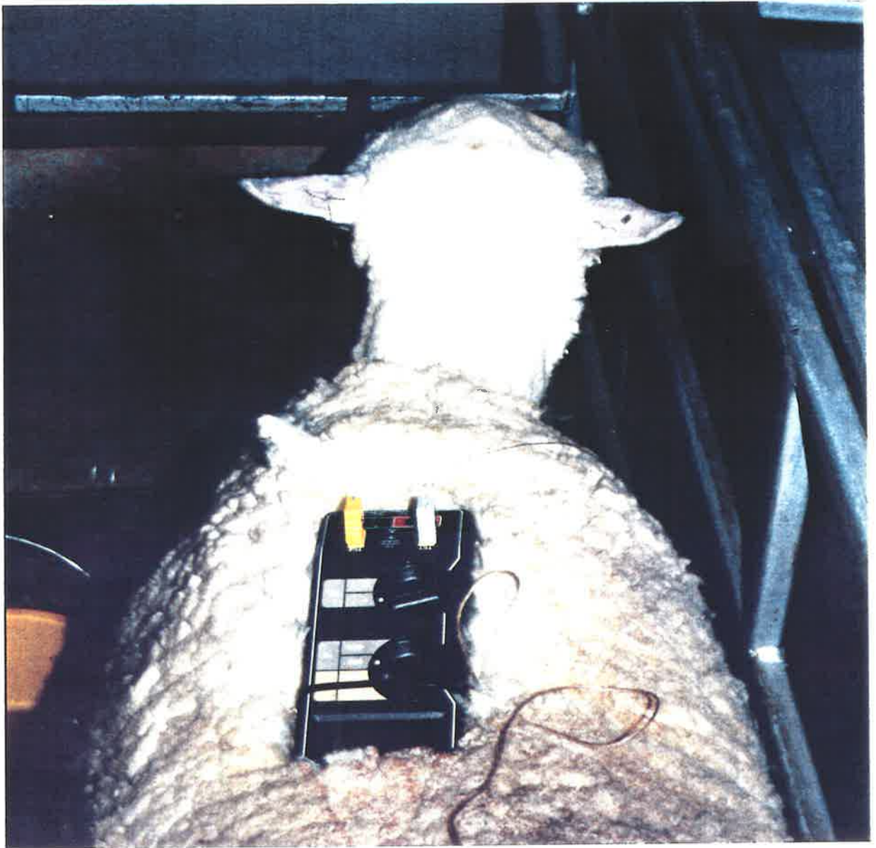
Plate 4.2. A Merino wether with a digital thermometer mounted on its back to record ear temperatures during environmental cooling.
