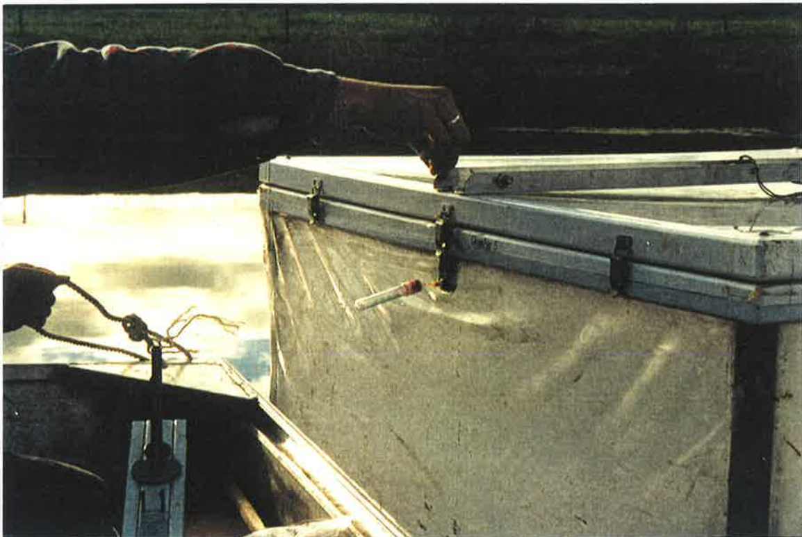
Figure 3.7: A detailed view of gas sample extraction from a static chamber using an evacuated tube and a hypodermic needle.
