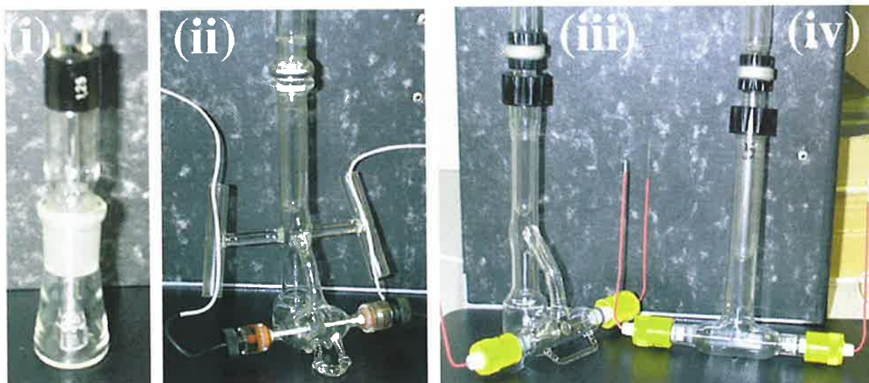
Figure 2.3: Cell types (i) The Philips PW95 series cell, (ii) cell designed and constructed by the Shiner group, The University of Indiana, (iii) cell designed and constructed by the Taylor group, The University of Adelaide, including a stirrer bulb and (iv) simplified cell design from the Taylor group, The University of Adelaide.
