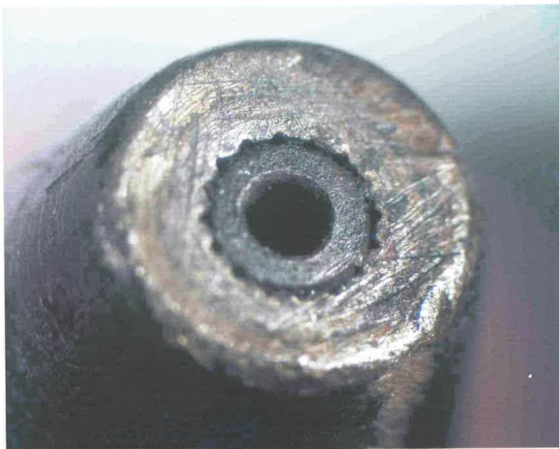
Figure 6: Tip of the modified glass-blowing burner used in the imaging experiments.
