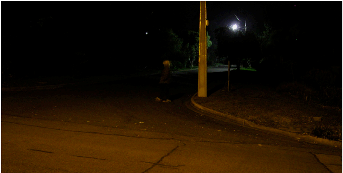
Figure 2.4 View of a pedestrian through the front side window: 35% VLT tint film
