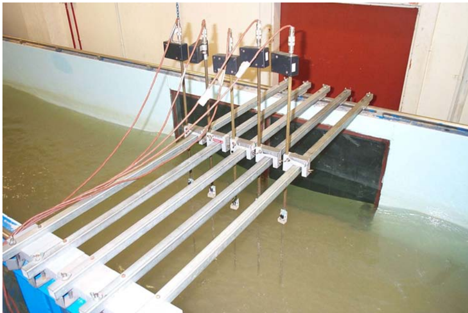
Plate C.4 The setup of the directional array for the wave reflection tests.
