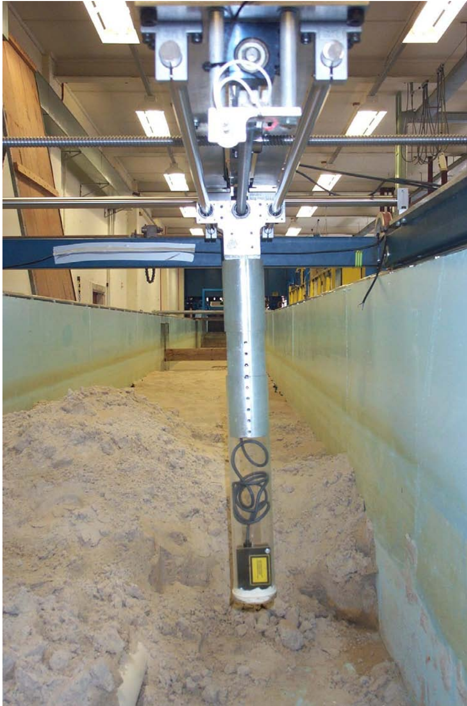
Plate E.2 The primary carriage of the ripple measurement system.
