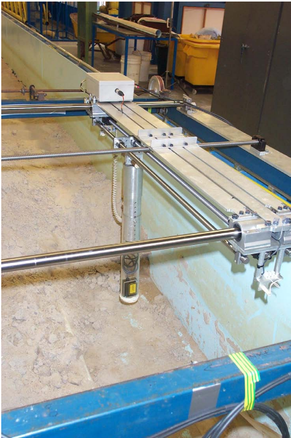
Plate E.5 The top view of the ripple measurement system.
