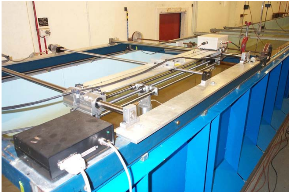
Plate E.1 The X-Y positional table of the ripple measurement system designed and developed by this study.
