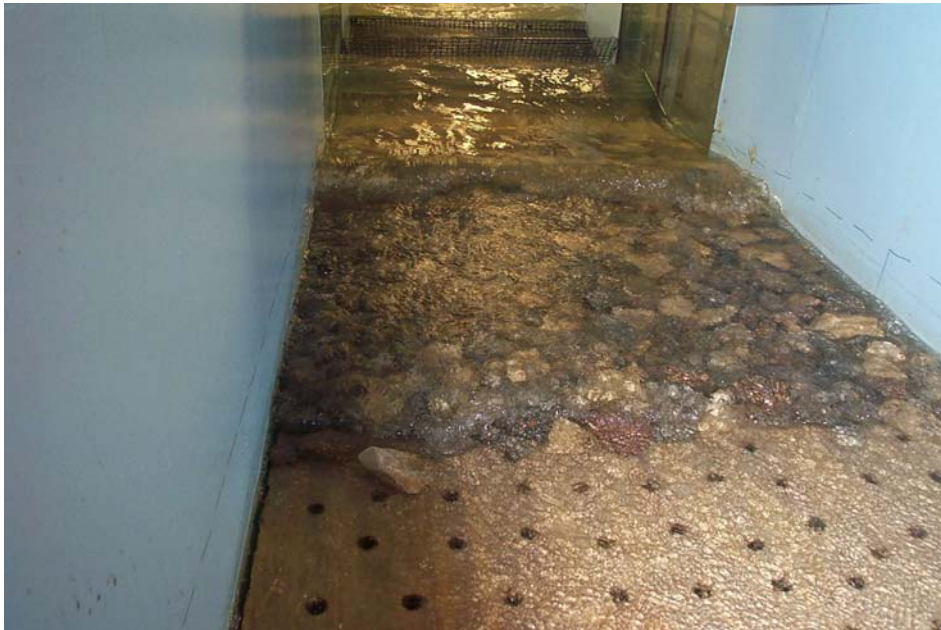
Plate C.3 Wave dissipation beach from the back.
