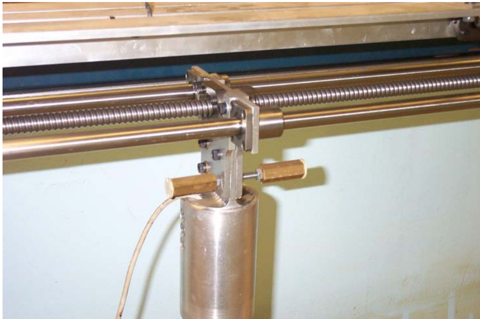
Plate E.6 The primary carriage of the ripple measurement system.
