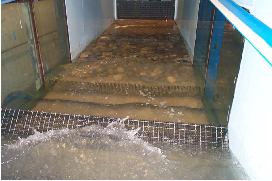
Plate C.1 Wave dissipation beach from the front.
