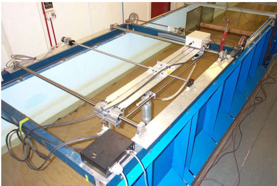
Plate 3.1 The X-Y positional table of the ripple measurement system designed and developed by this study.
