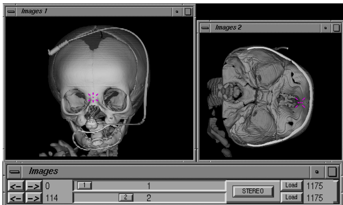
Figure 3.7 Two reconstructed 3-D images are displayed by default as shown. Image 1 is the model interpolated from the set of Z-axis views. A ‘movie’ set of images can be run to show the picture rotating. Image 2 is the model interpolated from the X-axis views that can also be rotated.
