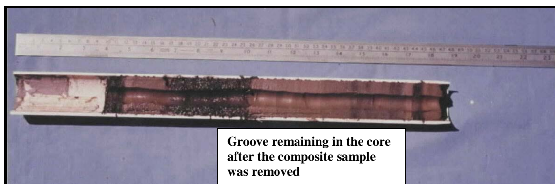
Figure 3.5: Composite sample removed from tailings core – Site 4 (9-9.5 m)
