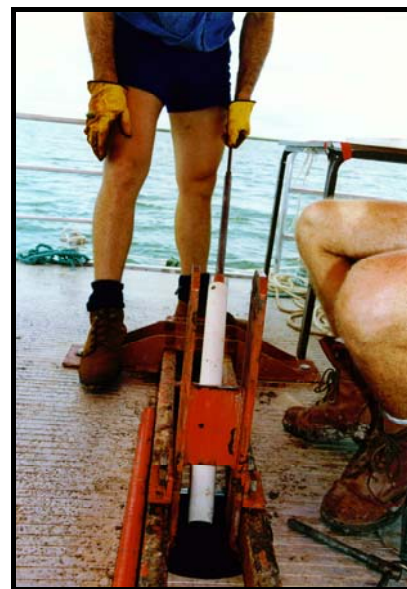
Figure 3.3: UPVC sampling tube
