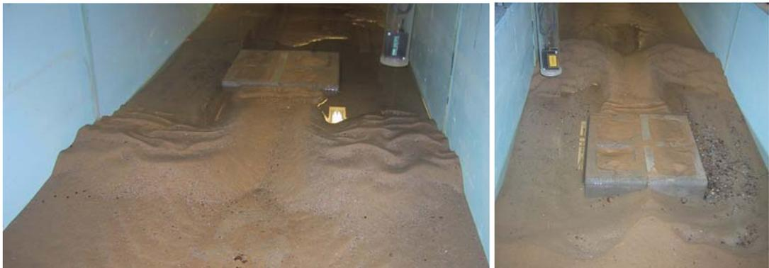
Figure 3.26 The resultant morphology in the channel from Experiment One, looking upstream and downstream respectively. The water and upper parts of the obstruction have been removed.
