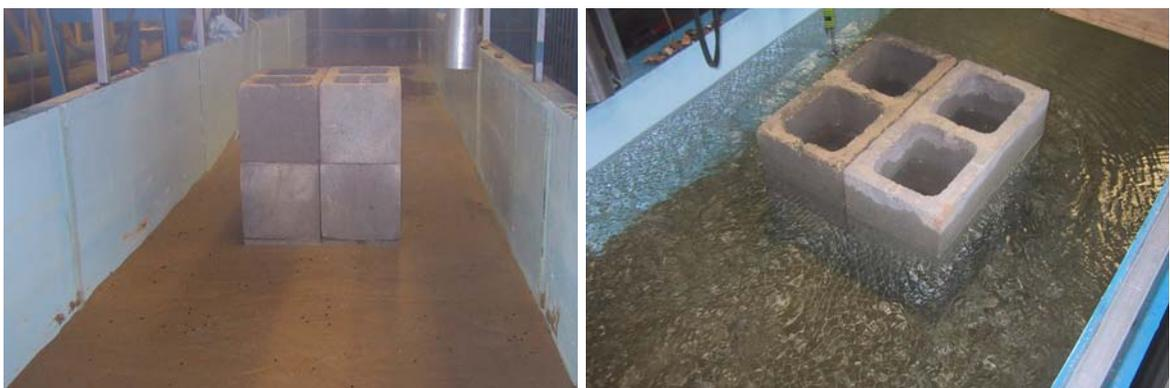
Figure 3.23 The obstruction in the rectangular flume, before and during experiments.
