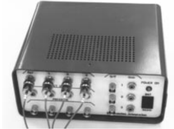
Figure 3.35: The signal conditioning unit housing the microphone amplifiers and differential amplifiers used to calculate mean pressure and particle velocity for three axes.
