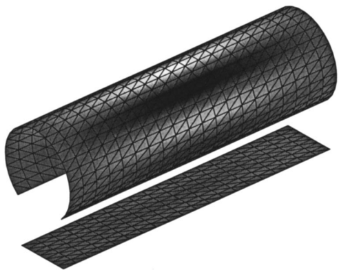
FIG. 11. Mode shape of the third normal structural mode (33 Hz).
