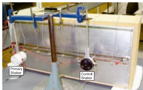
Figure 4.37: Photograph of the experimental apparatus used to predict the performance of the energy density sensor as an error sensor.
