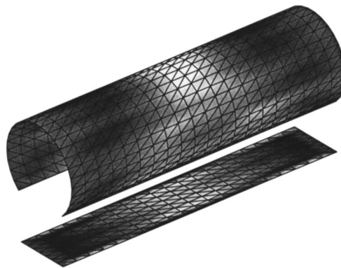
FIG. 8. Mode shape of the most efficient radiation mode at 117 Hz.
