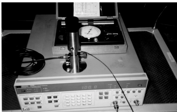
Figure B.1 Configuration of UA0914 sound intensity coupler for calibrating electret microphones
