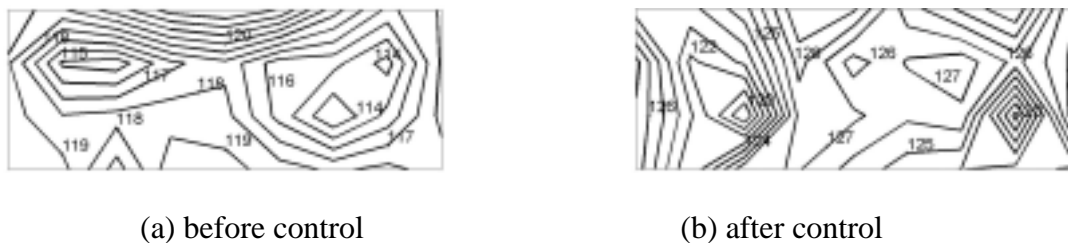
Figure 6.18 Distribution of velocity level on the transformer tank (top panel) corresponding to the minimization of the sum of the squared sound pressures using 8 control sources and 8 error sensors, at 100 Hz
