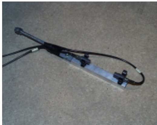
Figure 6.4 A photograph of the sound intensity probe constructed by two electret microphones
