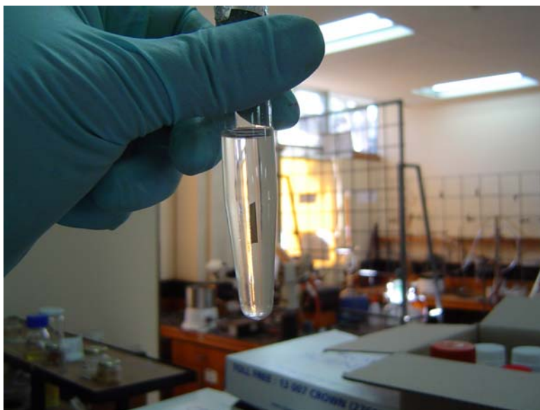
Figure 3.2: Wafers placed in SBF in vertical direction.
