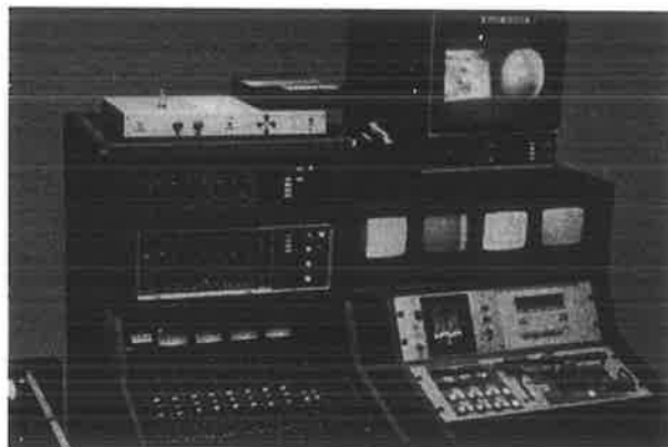
FIG. 3. Video and audio control console, with a high-resolution colour video monitor and the 1-in. videotape recorder/reproducer on the left. The special processing unit is placed on the top of the control console.
