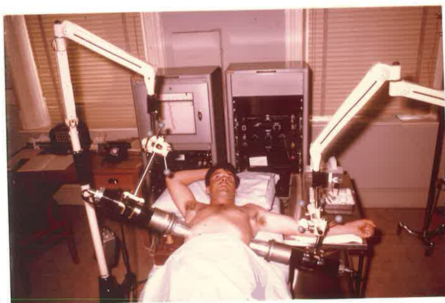
Figure 2: Recording organ count rates with shielded scintillation probes over the surface markings of liver and spleen.
