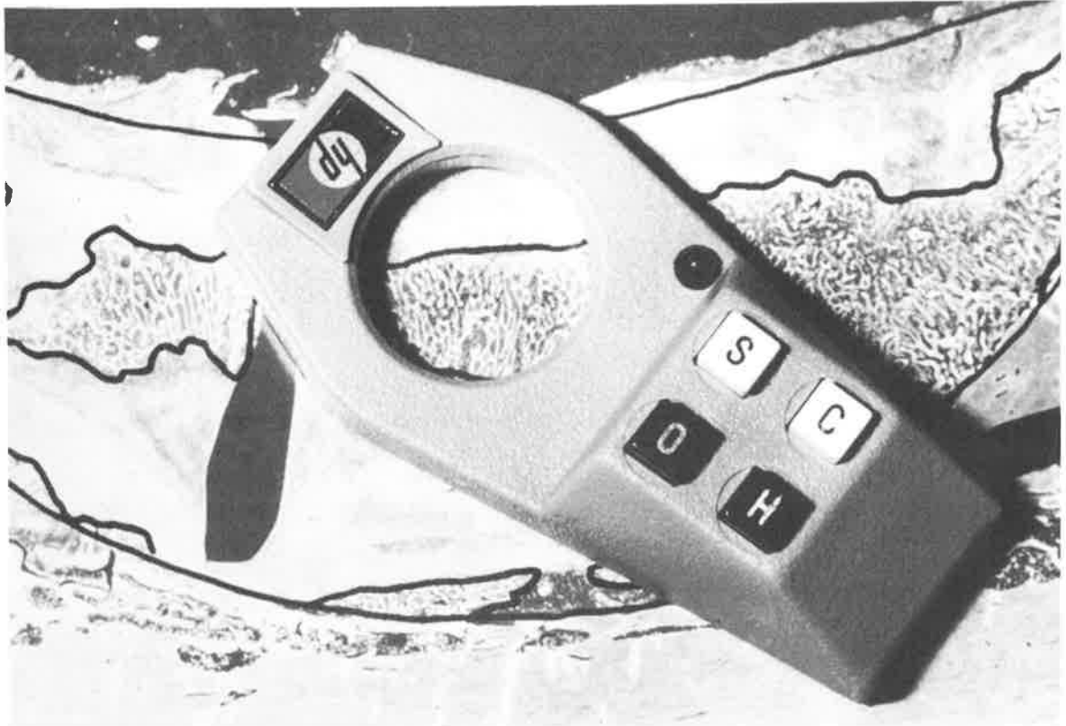
Fig. 6.11 The cursor of the Hewlett Packard digitizer in position on an enlarged photograph of the defect in which the outline of the defect and areas of new bone have been emphasized with black lines
