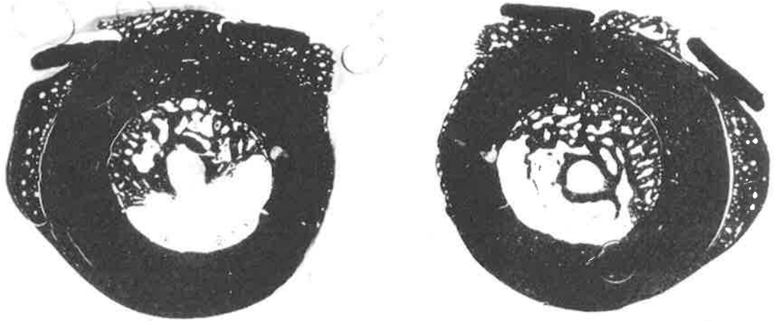
Fig. 8.17 A thin plate specimen at 12 weeks showing similar bone formation in the medium holes with both active (left) and inactive (right) stimulators
