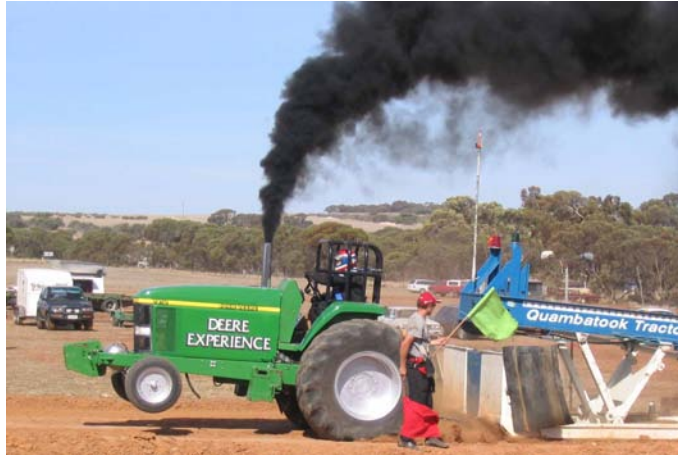
Figure 2.4: Example of soot emission
