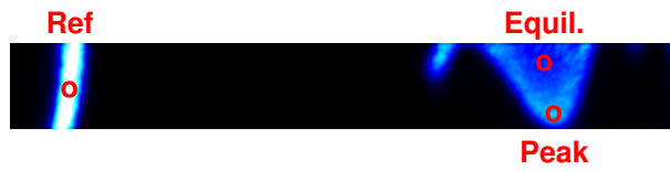
Figure 3.29: Image of slot burner reference flame (left) and premixed flame front (right)
