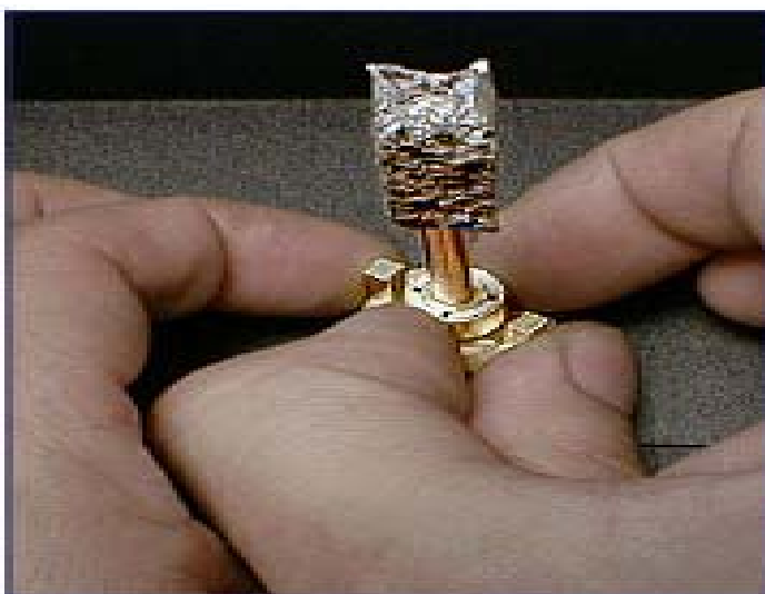
Figure 8: Special specimen holder 4 mm in diameter
