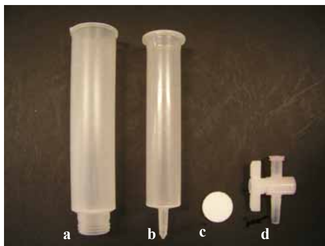
Figure 7.4. Equipment for sepharose CL-4B chromatography, (a) reservoir, (b) PD-10 column, (c) frit, (d) stopcock.
