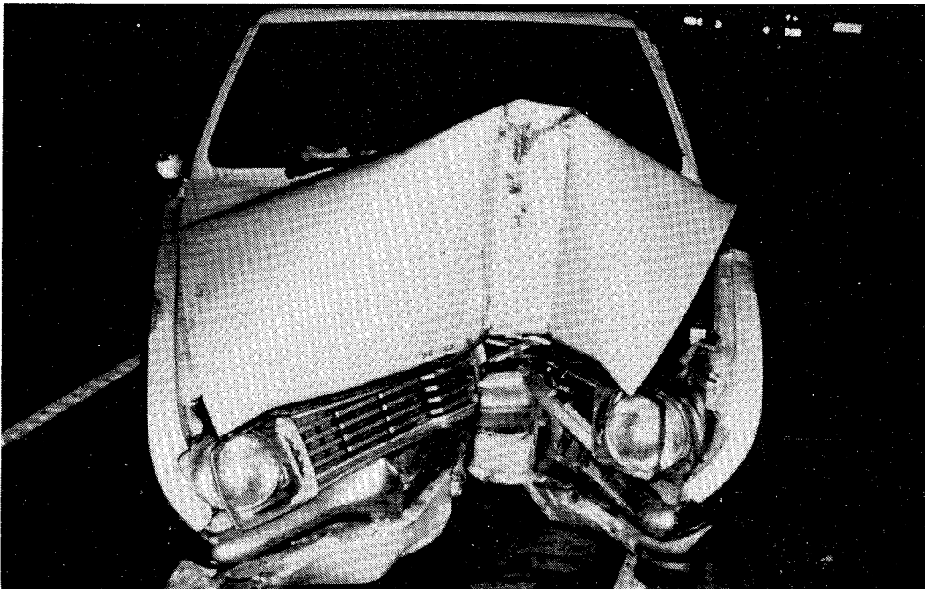
FIGURE 4.27: Damage to car involved in frontal impact with utility pole (Accident 096, See Figures 4.28, 4.29)
