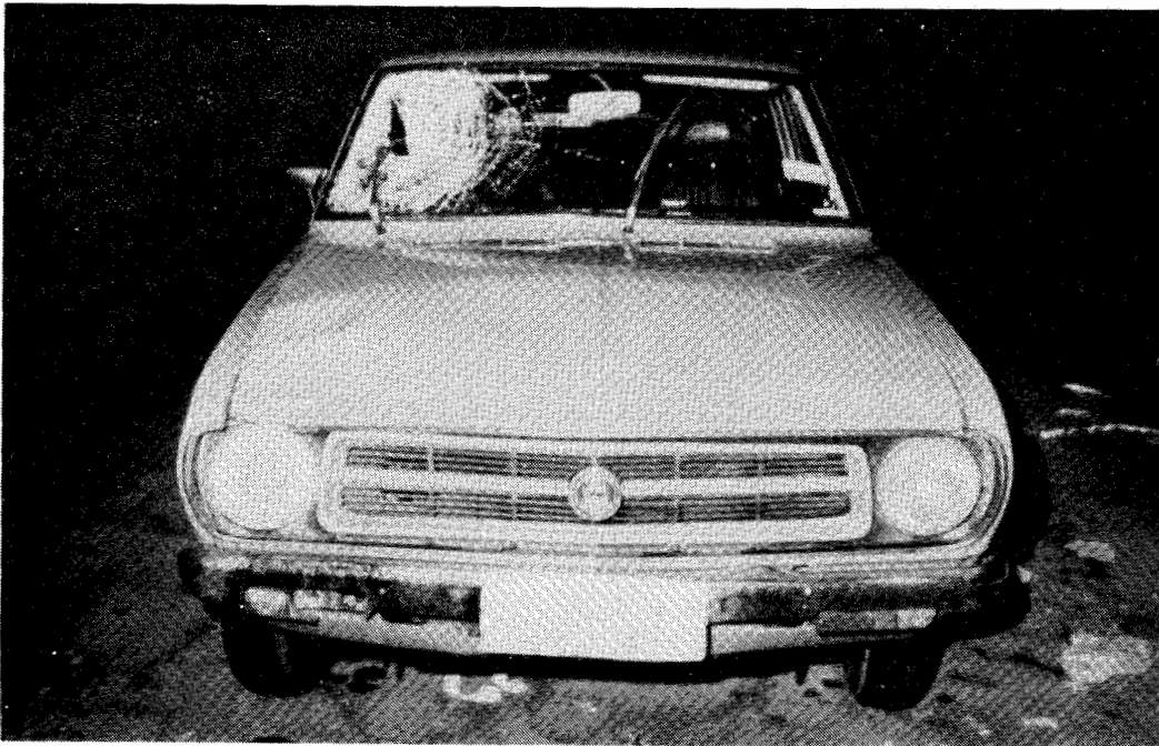
FIGURE 4.41: Datsun 1200 following impact with pedestrian. (Accident 144, See Figures 4.42, 4.43)
