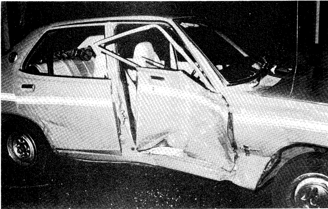
FIGURE 4.7: Damage resulting from a two-car collision. Note separation of door latch (Accident 230, see also Figures 4.8 to 4.11)
