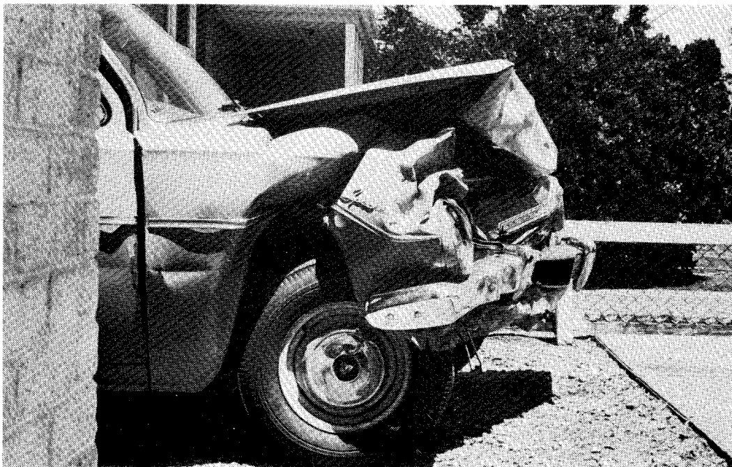
FIGURE 4.81: Damage resulting from a head-on collision (Accident 245, see Figures 4.82 and 4.48 et seq.)
