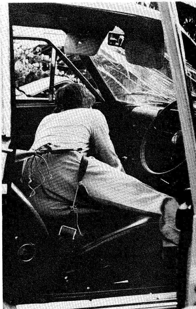
FIGURE 4.22: Approximate position of driver following rearward movement of seat back in rear impact (See Figures 4.19 to 4.23)
