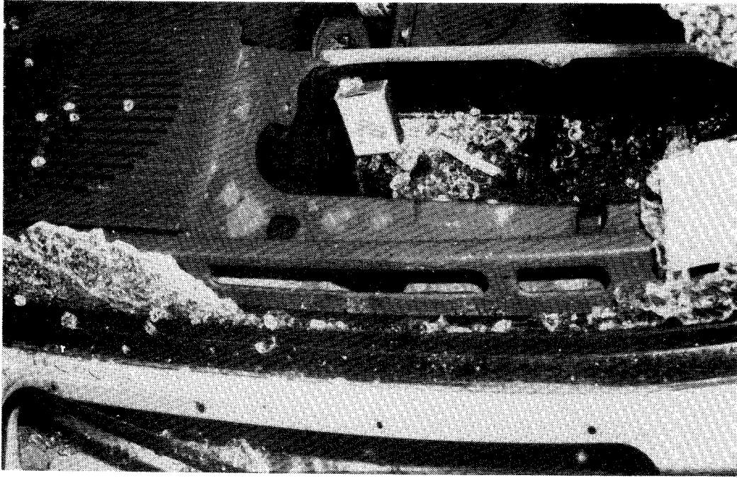
FIGURE 4.34: Lower edge of windshield frame and retained fragments of shattered toughened glass struck by face of unrestrained front seat passenger (glove box lid is open and grill is missing from plenum chamber in front of the windshield) (Accident 121)
