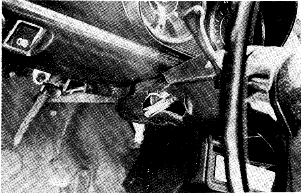
FIGURE 4.84: Damage to plastic housing around steering column from impact by driver's knee. (1970 Fiat 125S sedan, Accident 008)
