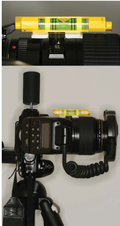
Figure 22. Fluid level used to calibrate camera lens to true horizontal
