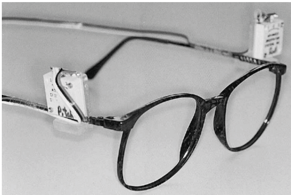
Figure 18. Two inclinometers for pitch and roll fixed to a pair of spectacles 83
