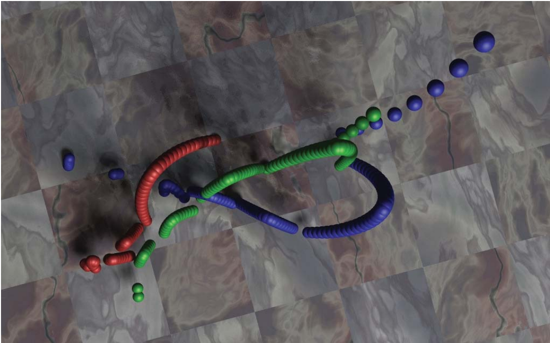
Figure 5.7: A reconstruction of 3D ball trajectories, projected to virtual cameras, for matches identified by CATSAC assuming an unknown frame rate ratio
