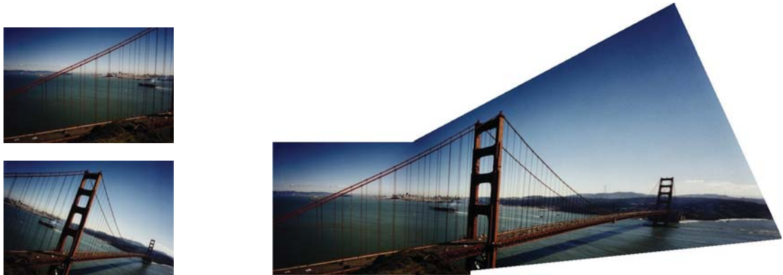
Figure 2.4: An application of the homography matrix; original images and the resulting mosaic
