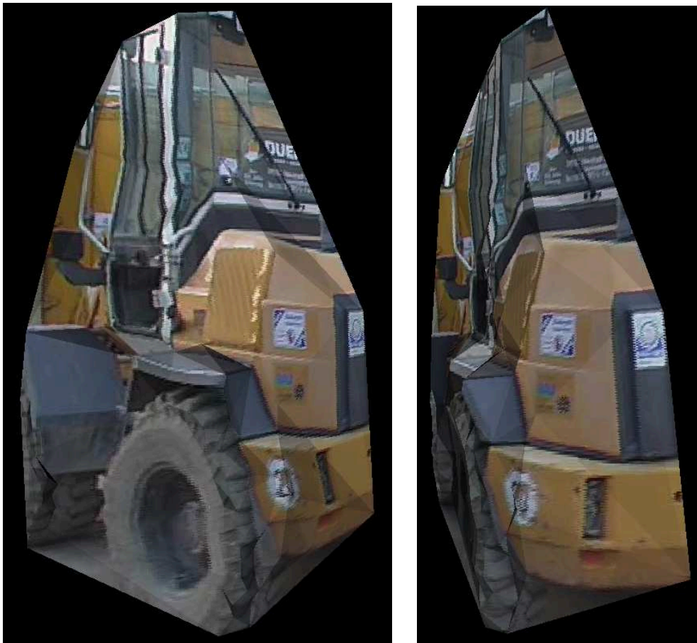
Figure 5.11. Two views of the 3-D model obtained from the RFNS-TGN trifocal tensor estimate.
