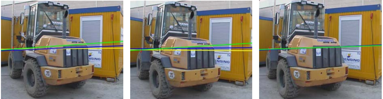
Figure 5.12. An example of epipolar lines for a particular data point. The blue and green lines are obtained from fundamental matrices retrieved from the NALS and RFNS-TGN trifocal tensors respectively and the yellow lines are from GS. In this case all three lines are distinct except in the third view where they are grouped closer together.
