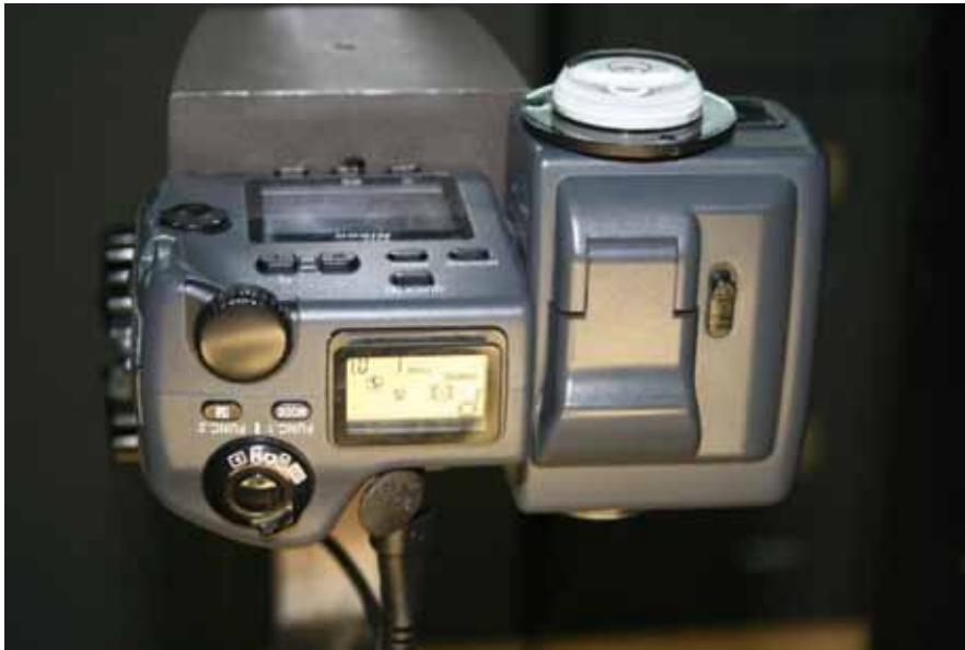
Figure 12: Spirit level used to ensure camera is leveled.
