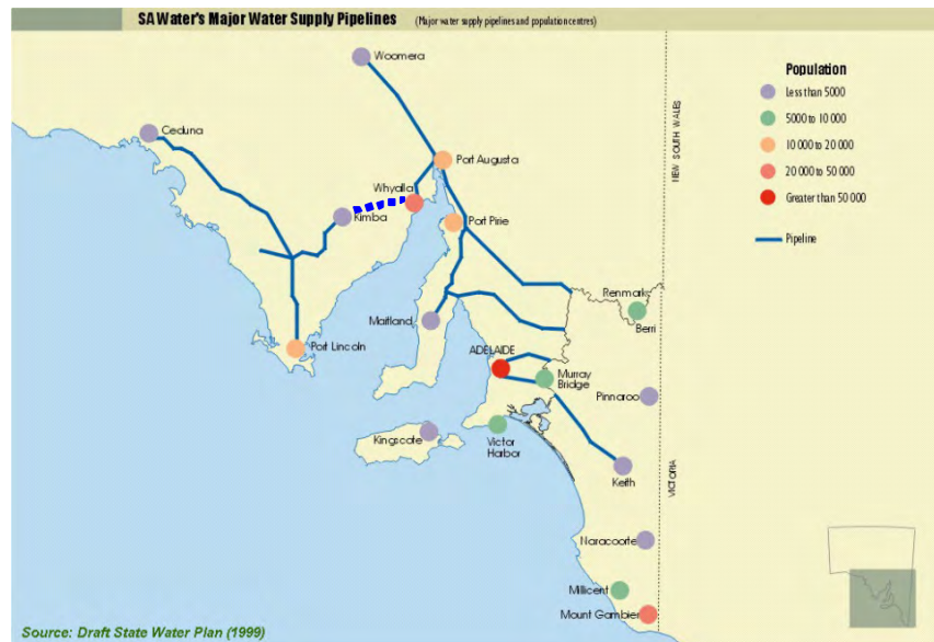
Figure 55 Major Water Supply Systems South Australia (SWP 1999)
