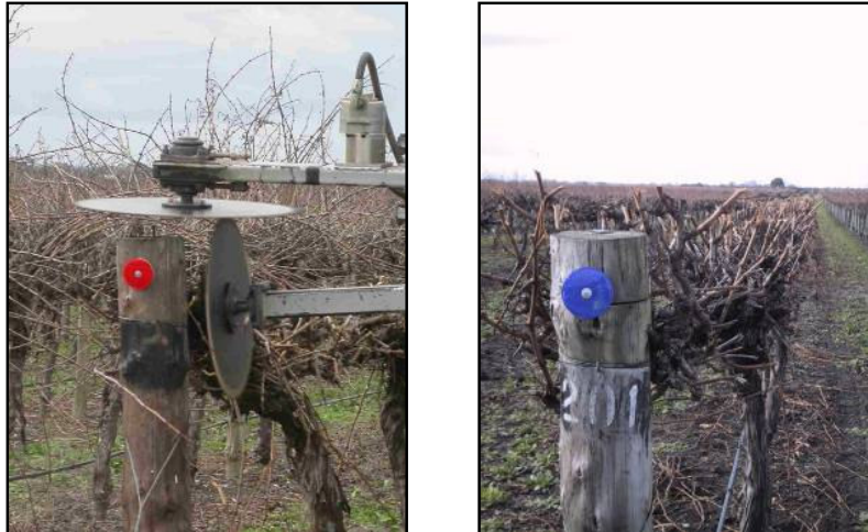
Figure 3.16 Mechanical hedge saw pruning: Vitis vinifera cv. Cabernet Sauvignon vines at Coonawarra (2005) pre-pruning (left) and post-pruning (right).
